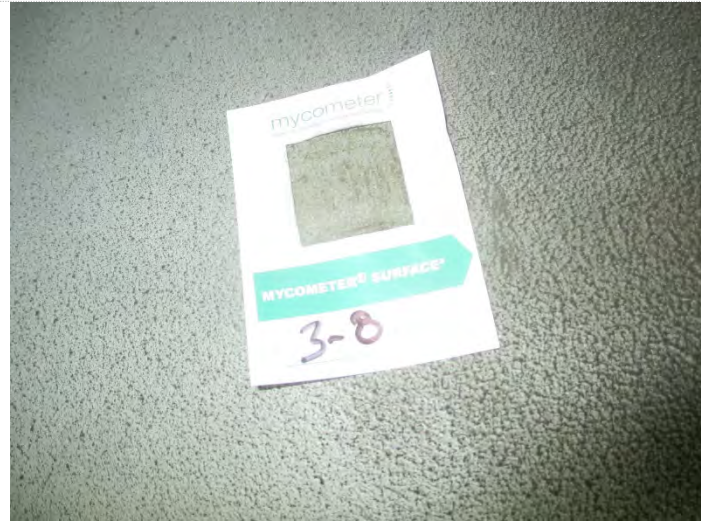
Photo 13: Sample # 3-8: VAV F3-3, Rm 108 Internal side; MSFV= 59, Old inactive Mold Growth Category IV Aspergillus/Penicillium and Chaetomium
